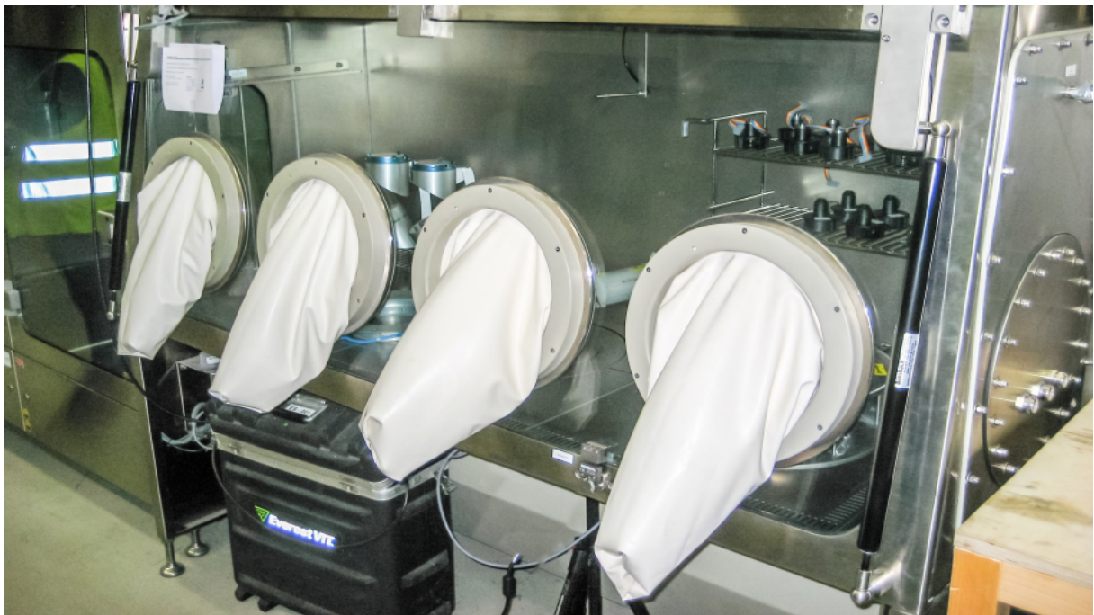
Figure 1: MAS-100 NT viable air samplers in a PSI (SKAN AG 2019) from SKAN AG (photo courtesy of SKAN AG)
